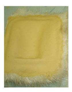
These laminates should change from a brown colour to a creamy colour, indicating the onset of cure. If further thickness is required this may commence once the initial laminate has cooled completely.
