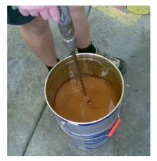
An air motor fitter with a mixing blade should be used to mix the filler back into suspension. This essential step takes about 10 minutes.
