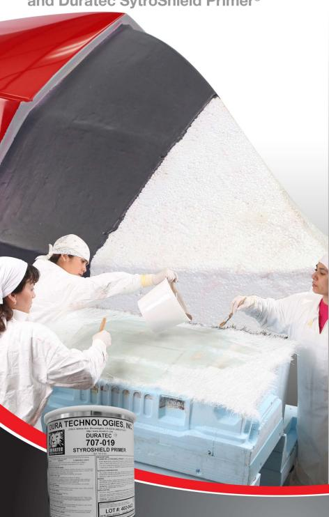
For use with Expanded Polystyrene Foam (EPS). Use low-cost EPS in place of Urethane tooling board or MDF for fast, economical patterns, shapes and decorative features.
